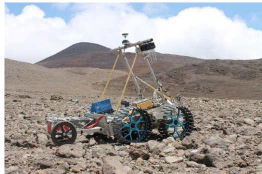
Figure 29. Juno II rover with MMAMA instruments traversing in Apollo Valley
