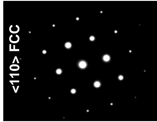
Figure 9.—MC carbide phase, FCC, Fm3m, a~4.3 Å: a. TEM image and b. SAEDP of LFW760-1k.
