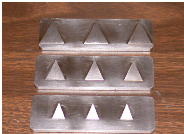
Figure 1.—Picture of three micro-ramp inserts from the experiment in the 15- by 15-cm supersonic wind tunnel.
