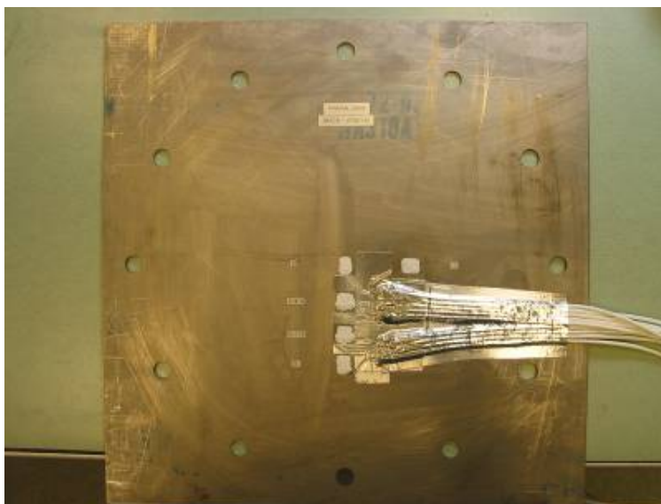
Figure 1.—Plate test specimen with strain gages mounted on the rear face
