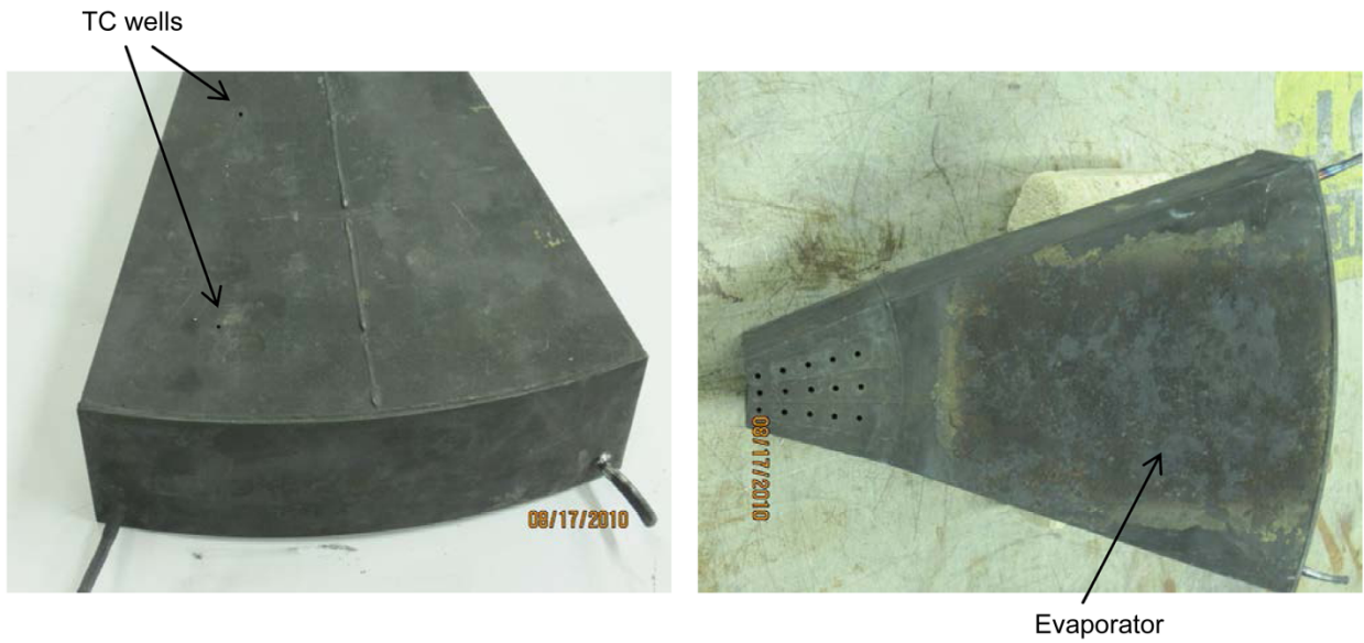
Figure 3.—Heat pipe at the end of life testing.
