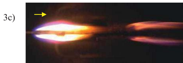
Figure 3: Visible flame images of the flame at the end of the test. a) edge view; b) front view; c) test at 35% O 2 , 20 cm/s with fully separated flames. Arrows indicate flow direction; dashed line indicates the incipient flame separation.
