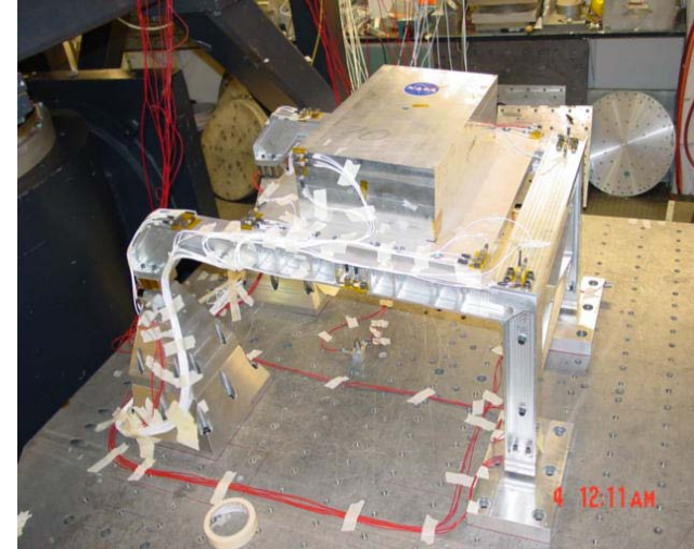
2) Small Pallet 70lb mass, hard mounted
