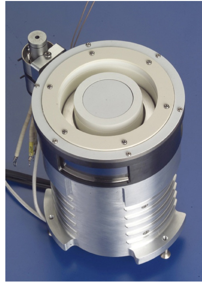
Figure 5 – HIVHAC laboratory thruster
