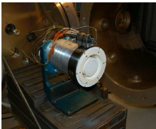
Figure 6 – HIVHAC thruster installed for extended wear test
