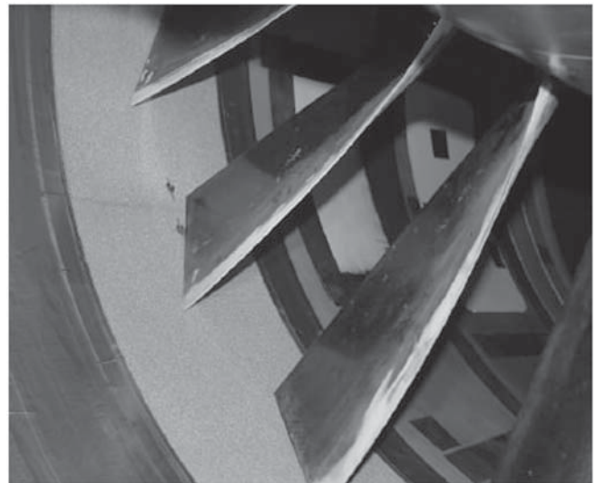
Fig. 11 FML spool installed over the rotor.
