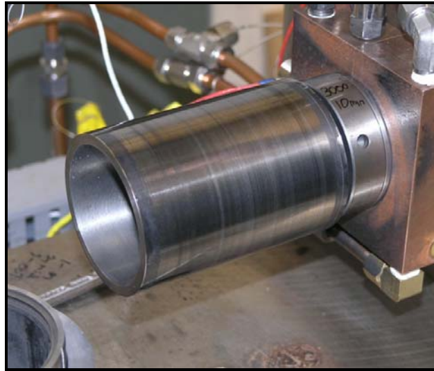
Figure 10. Condition of the PS304 coating after continuous sliding for 10 min while supporting 266.9 N. No spallation or delamination is evident.
