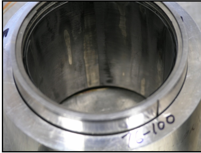
Figure 6. Bearing after 100 start-stop cycles showing removal of soft polymer from top foils.
