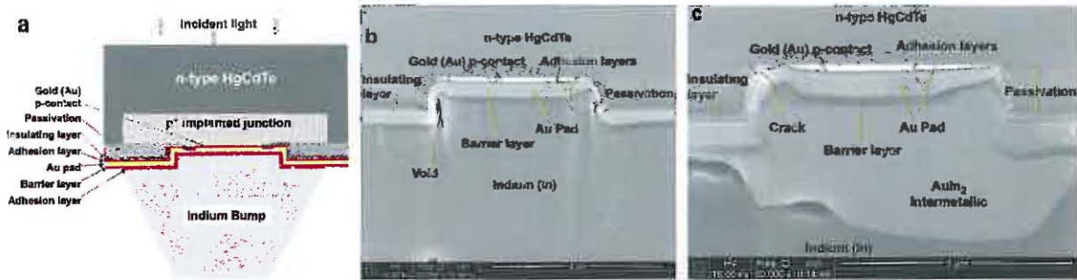
FIG. 4. a) Pixel contact structure; b) Scanning Electron Microscope (SEM) image of a non-degraded pixel in NIRCcam detector C105; c) SEM of degraded pixel in NIRCcam detector C094
