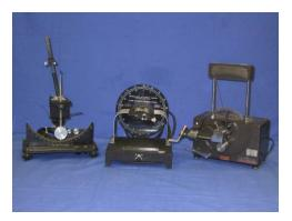
The Gurley Stiffness Tester measures the bending stiffness of textile and flexible materials. The applicable test standard includes ASTM D1388.
