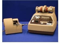
The Altas Accelerator is designed to rapidly determine wet and dry abrasion resistance of flexible materials, including textiles, paper, leather, and plastics. Material specimens are rapidly tumbled within a cylindrical test chamber lined with an appropriate abrasion material. The tumbling action is provided by a propeller-shaped rotor for a predetermined time at a predetermined speed. The applicable test standard includes AATCC Test Method 93.
