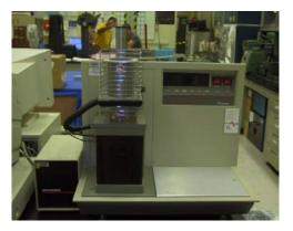
temperature range of -100 to 200 °C at an atmospheric pressure to  $1 \times 10^{-5}$  Torr pressure. This instrument is compliant with ASTM E2585.
