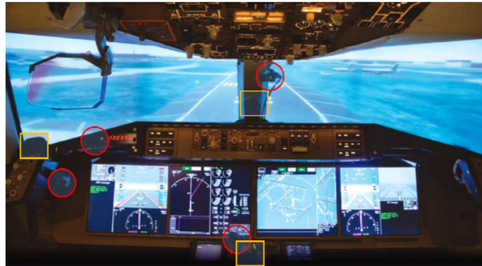
Figure 1. Camera and Illuminator Locations in RFD
