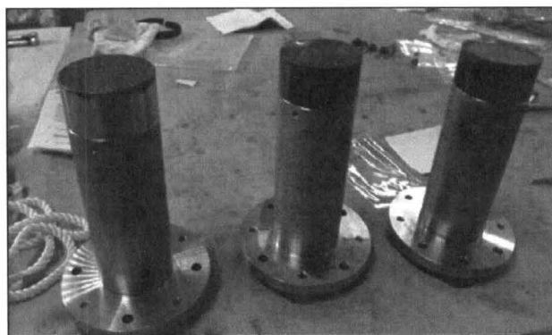
Figure 13. HY-80 witness rods ready for installation
