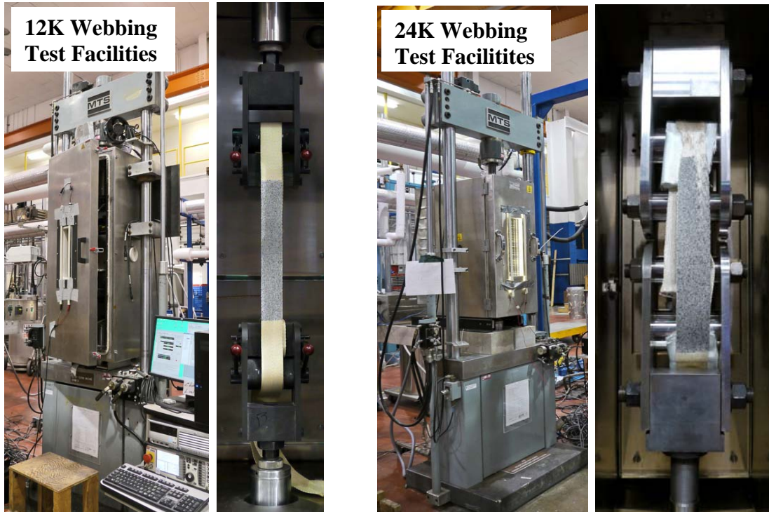
Figure A-1. MTS 55Kip load frames and grips for 12K and 24K creep testing
