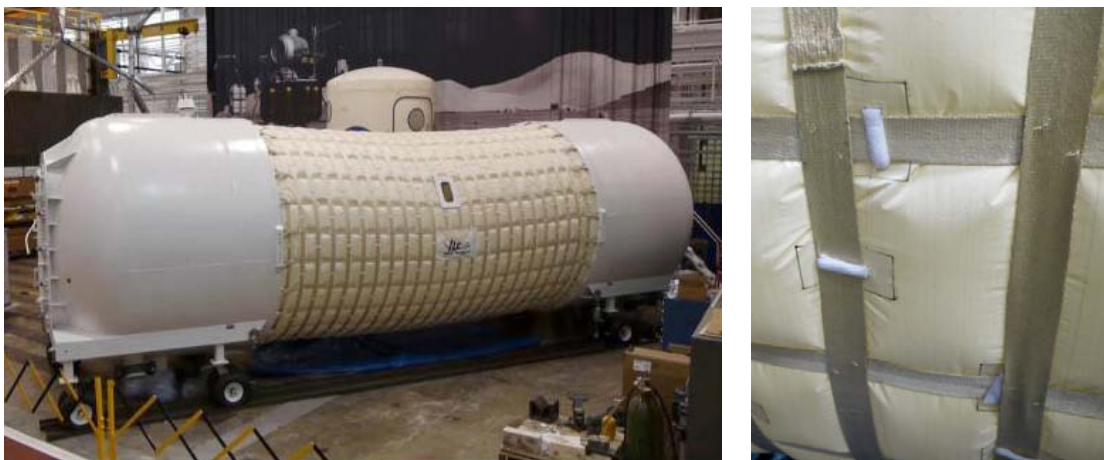
Figure 2. The expandable habitat EDU and a close-up of the Vectran webbing.
