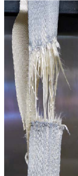
Figure 19. 12K 70% UTS stitched Vectran failure.
