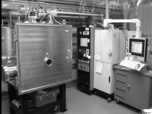
The L3-Tinsley NIBF (Narrow Ion Beam Figuring) system
