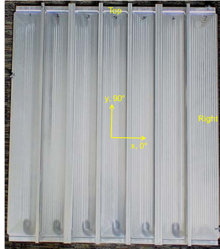
Figure 8. Picture of the stiffened side of the Al-2139 test panel.
