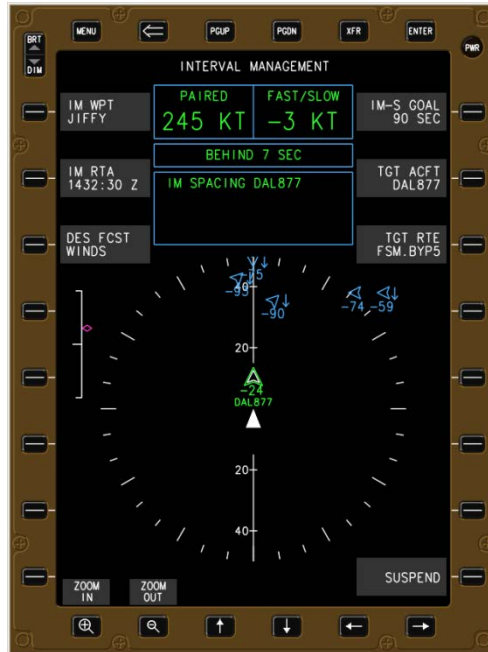
Figure 7. Electronic Flight Bag (EFB) with FIM clearance and traffic
