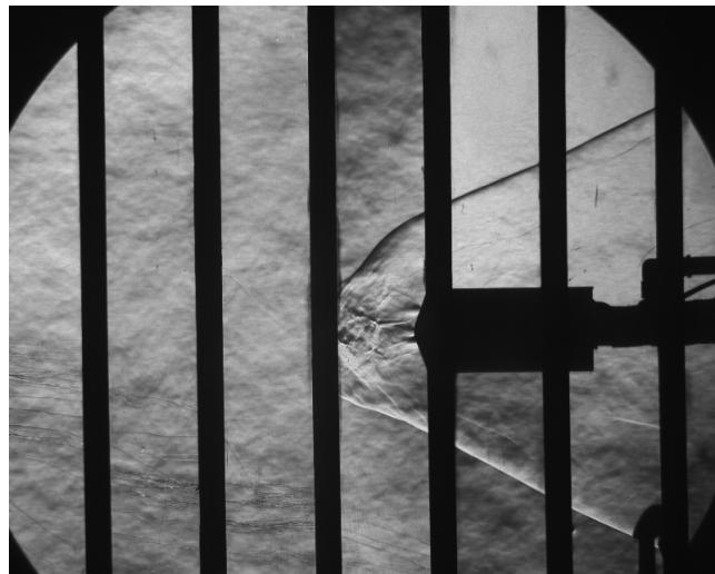
Figure 16 – Sample Schlieren result for quad-nozzle at Mach 4.6, \alpha = 0^\circ , \beta = 0^\circ , and C_T = 0.91
