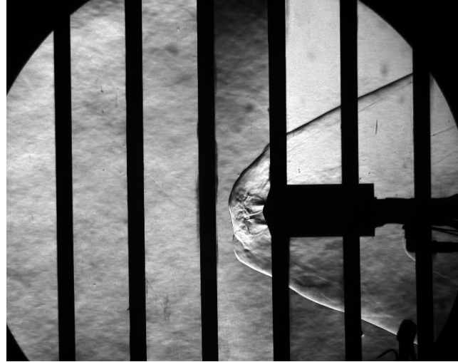
Figure 13 – Sample Schlieren result for tri-nozzle at Mach 4.6, \alpha = 0^\circ , \beta = 180^\circ , and C_T = 0.90
