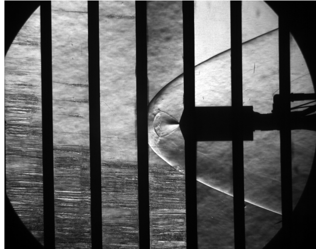
Figure 6 – Sample Schlieren result for center nozzle at Mach 4.6, \alpha = 0^\circ , \beta = 0^\circ , and C_T = 0.94
