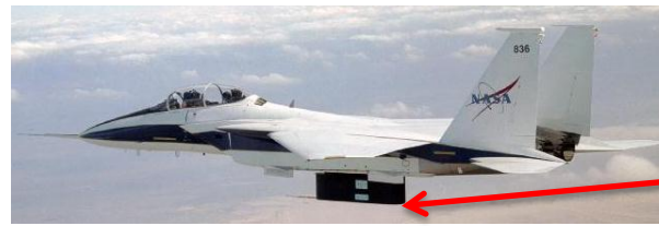
Leading Edge Stagnation Point (LESP) Tao Sensor Verification on ATW-II
