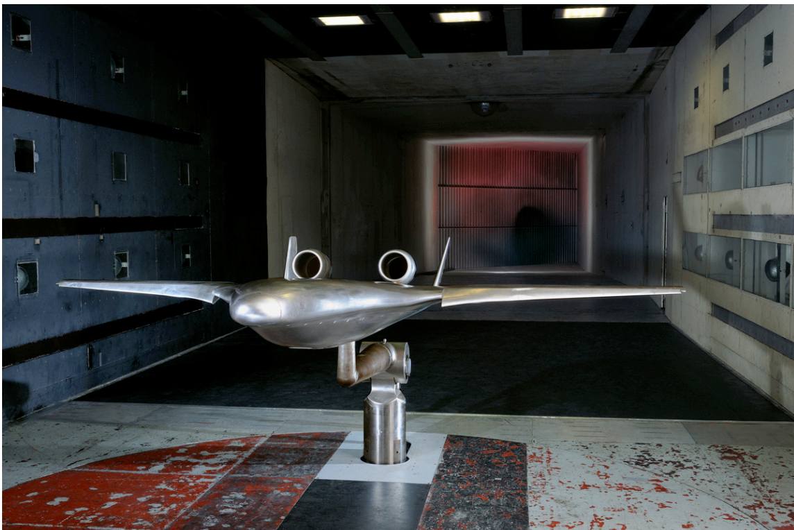
Figure 4. HWB model as tested in the NASA Langley 14- by 22-Foot Subsonic Tunnel.
