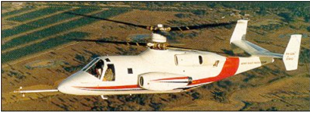
Figure 1. XH-59A coaxial lift-offset helicopter.
