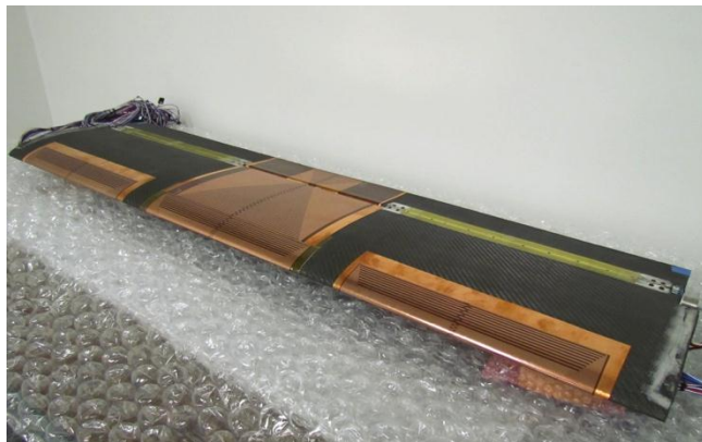
MUTT-like wing instrumented at three span stations
