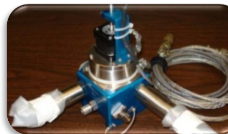
Figure 1. Early Variable Oxygen Regulator bench-top prototype.
