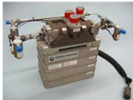
Figure 3. Rapid Cycle Amine Swing Bed Unit 1.0
