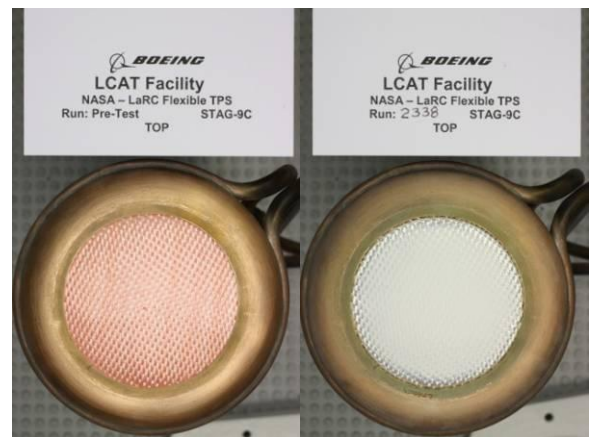
Fig 18: Left: a pre-test FTSP sample; right: post test.
