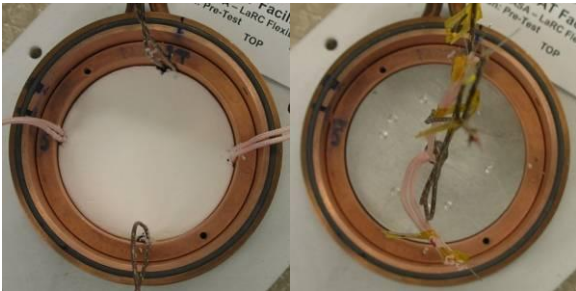
Fig 15: Left: backside insulator installed, right: support plate installed.
