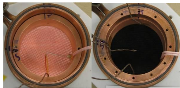
Fig 14: Installation of FTPS layers and thermocouples.
