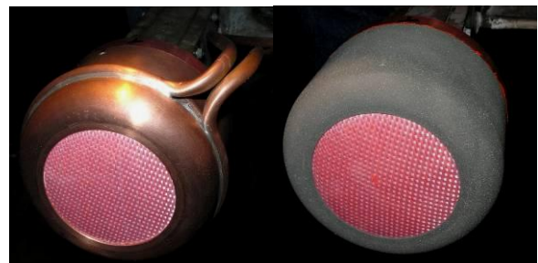
Fig 12: Stagnation model holders prior to a test; left: copper water-cooled version, right: SiC-coated graphite version.
