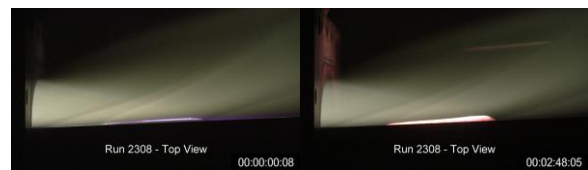
Fig 24: Testing of a FTPS sample with a mechanically locked boundary (initial model holder design); left: beginning of run, right: end of run (flow is left to right).
