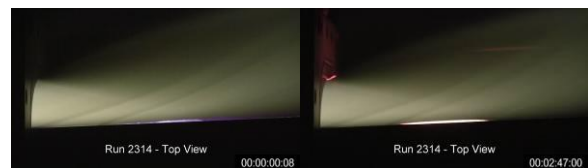
Fig 25: Testing of a FTPS sample with a mechanically free-floating, actively tensioned boundary (2 nd generation design); left: beginning of run; right: end of run (flow is left to right).
