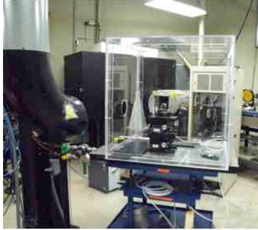
Figure 3. Plexiglass test box used to keep the test articles in a nitrogen-only environment
