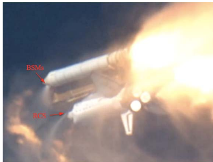
Figure 3. STS-117 SRB separation with BSM motors and RCS jets firing.
