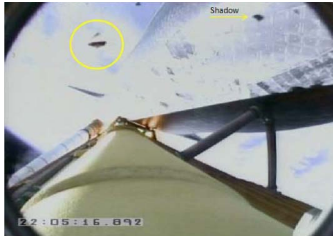
Figure 2. STS-127 TPS debris loss at MET=126 seconds (Ref. IIFA STS-127-I-004).
