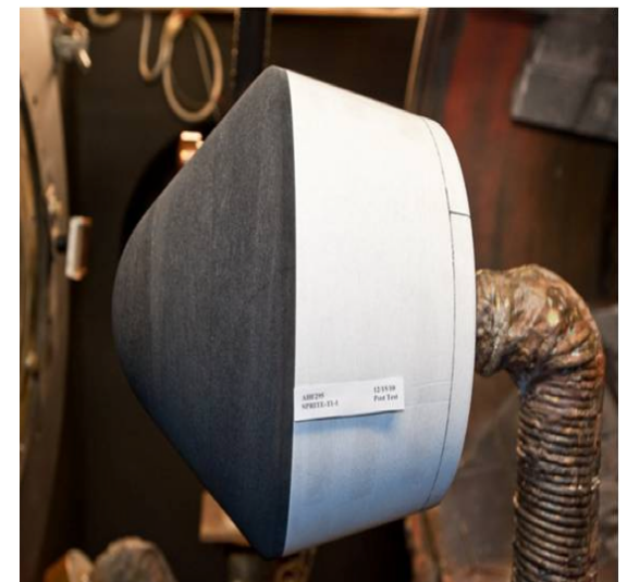
Post-Test Charred PICA Heatshield
