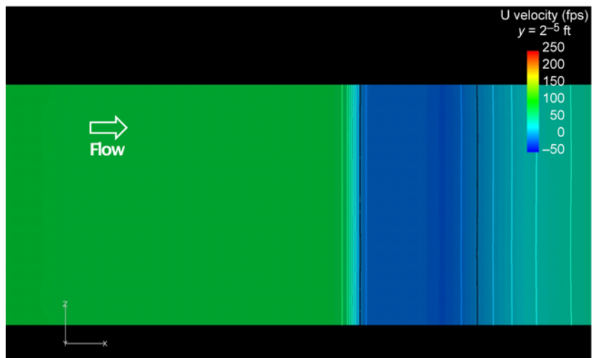
Figure 22.—Separation region in the baseline case as indicated by streamwise velocity component near the lower wall.
