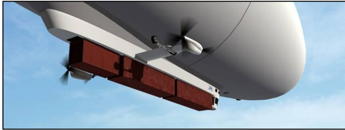
Airship with CONEX boxes
