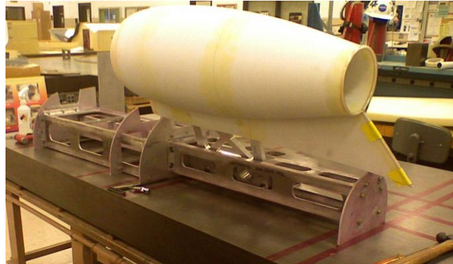
Figure 3. Flow-through engine nacelle and pylon bolted to aft fuselage skeleton.
