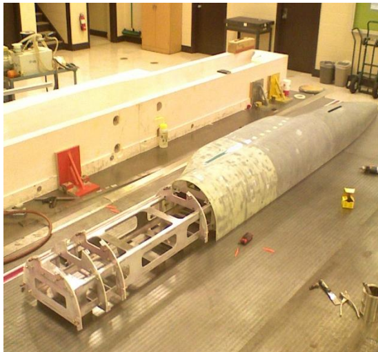
a) Aluminum ribs supporting composite skin
