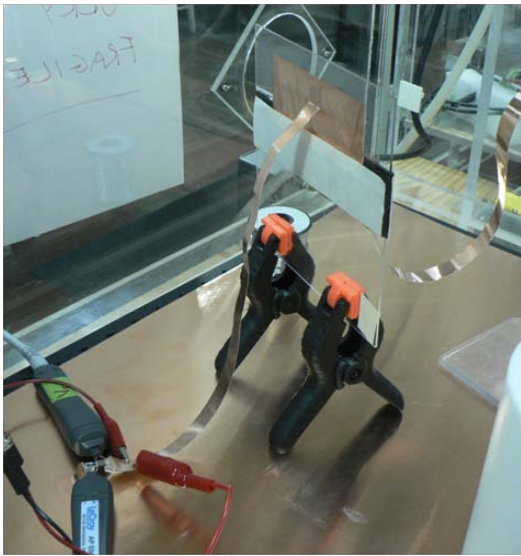
Figure 7. Experimental setup, showing actuator test article viewed from the covered electrode side, copper ground plane, flat copper tape leads, and capacitor-resistor assembly with differential probes attached. (Temporary red probes not used in final experiment)
