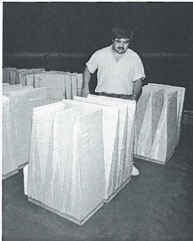
(b) Wedges used in coupon test in 40x80 test section.
