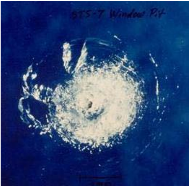
Figure 3. Space debris impact on Space Shuttle Challenger's front window on STS-7. [13]
