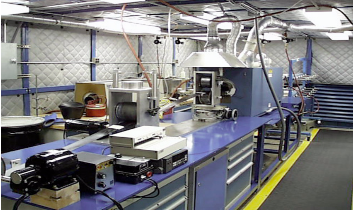
Figure 3. Langley dry tape processing line for thermoplastic polyimides.
