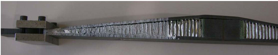
Figure 11. Photograph of the failed end of test coupon with clamped ends
