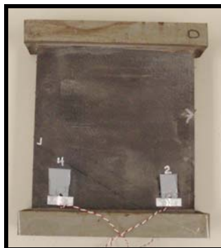
Figure 2. Front-view photograph of potted EWC and/or CAI test coupon.
