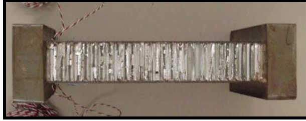
Figure 3. Side-view photograph of potted EWC and/or CAI test coupon.
