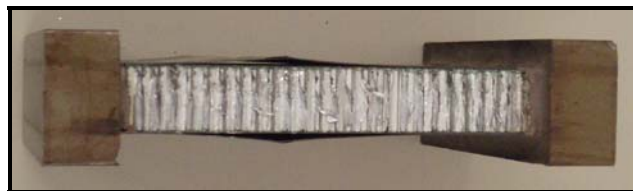
Figure 9. Photograph of ETW EWC from MTP-6003 showing typical valid failure mode including facesheet delamination and outward buckling on both the convex and concave sides.
