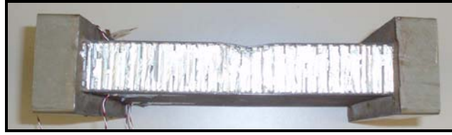
Figure 10. Photograph of ETW CAI from MTP-6010 showing typical facesheet buckling and core crushing valid failure mode.
