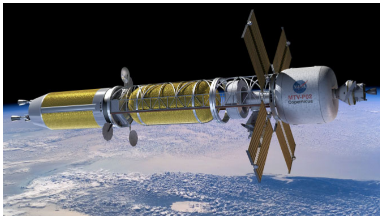
Fig. 1: Crewed NTR Mars Transfer Vehicle Allows NEA Survey and Short Orbital Stay Mars Missions.
