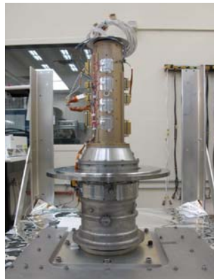
Figure 9. SMA mounted in test fixture to prepare for acceptance test in the clean room.
