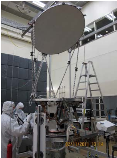
Figure 16. GMI Instrument during initial SMA Spin testing in Cleanroom with the reflector deployed
