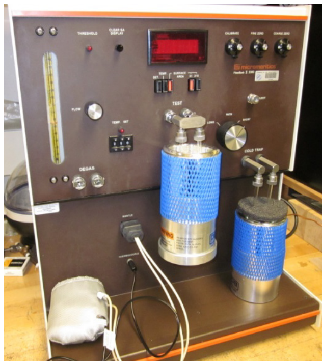
Figure 5.—Micromeritics FlowSorb II 2300 used for BET analysis.
