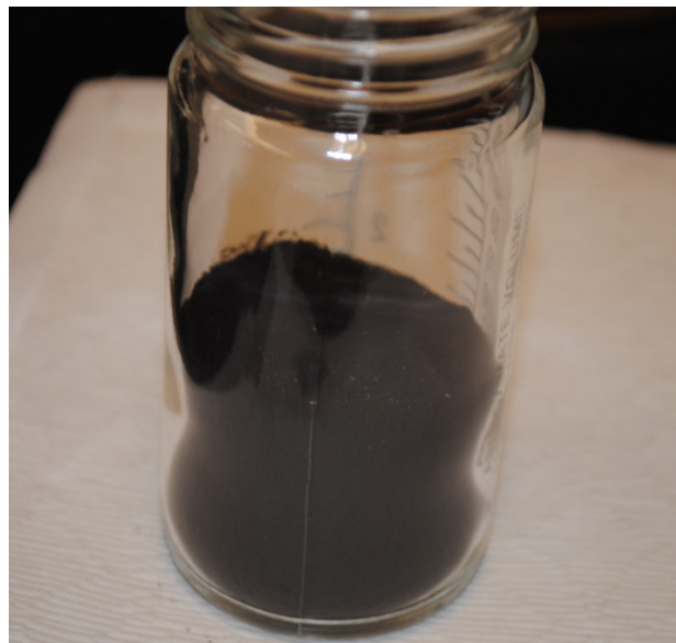
Figure 3.—Completed catalyst after calcination. Promoted and unpromoted catalysts both are black powders upon completion.
