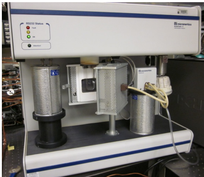
Figure 4.—Micromeritics AutoChem II 2920 used for TPR analysis.
