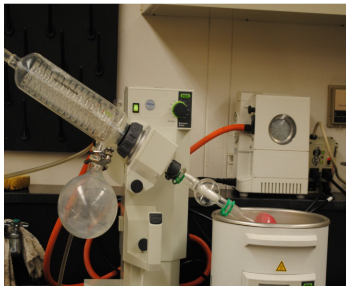
Figure 2.—Catalyst drying before calcination on Rotavapor 210.
