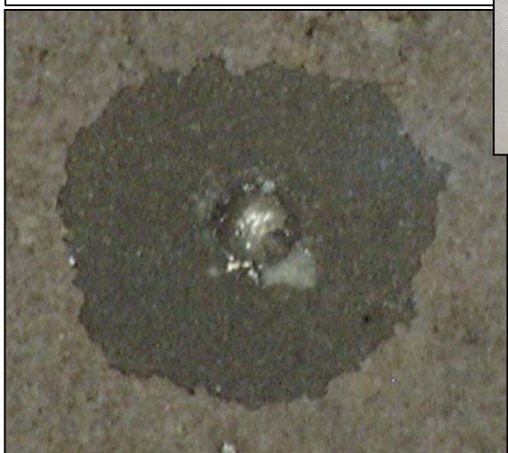
MPLM grapple fixture coating spall dia. = 0.6 mm
