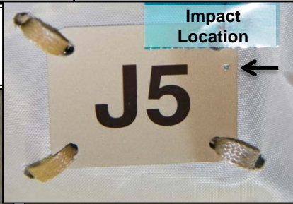
MPLM grapple fixture coating spall dia. = 0.6 mm
