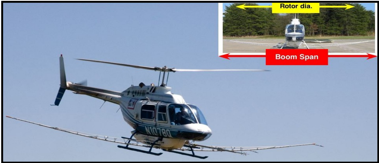
Fig. 2. The Bell 206B during the 2006 flight test program, configured with the inflight microphone array.
