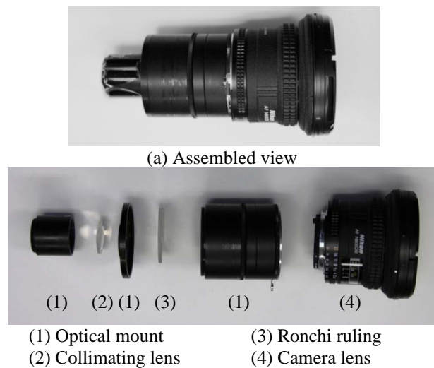
(b) Disassembled view Figure 4. Projector assembly.
