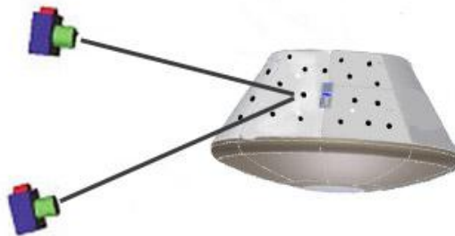
Figure 3. High contrast targets visible from multiple perspectives are required for accurate photogrammetric measurements.
