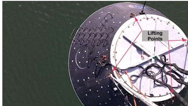
Figure 4. MLAS Crew Module with identified symmetric lifting points
