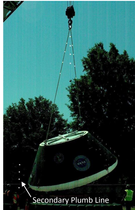
Figure 6.b Typical image from recorded sequence. Stationary plumb line visible to the left of the CM. Retroreflective markers on lifting strap highly visible in daylight conditions.
