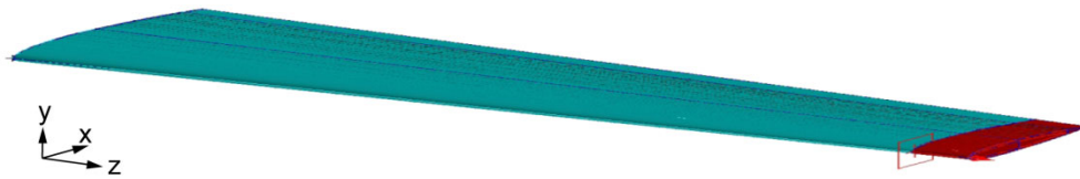
Figure 14.—Composite turbine hollow blade with solid cap.
