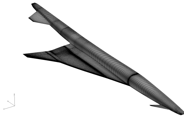
(a) CFL3D surface grid.
