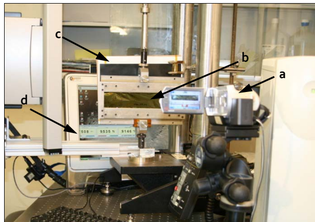
Figure 11. Arrangement of a) camcorder, b) mounted specimen, c) contrast screen and d) digital display
