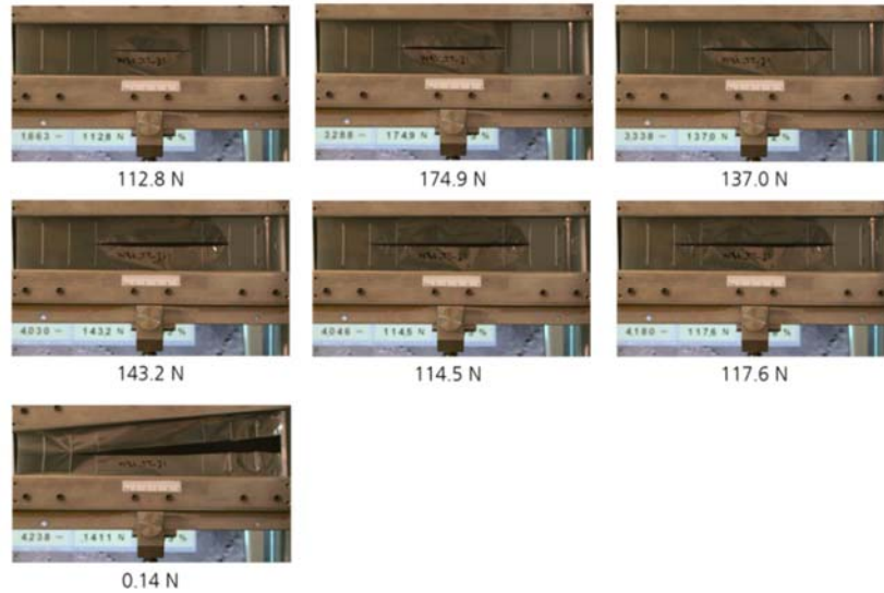
Figure 14. Sequence of a Rip-Stop Line specimen images and under displacement control
