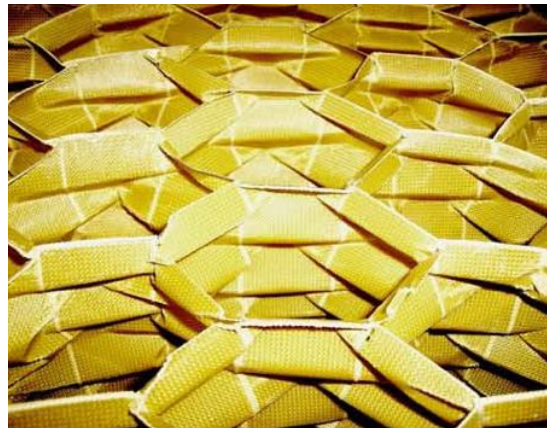
Figure 2. Close-up photograph of the crushing modes exhibited by the DEA.
