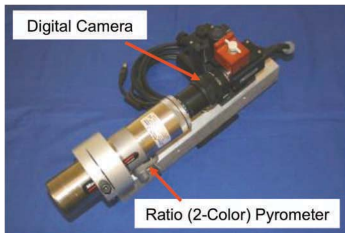
Figure 7. Photograph of digital camera and 2-color pyrometer used in HyMETS.
