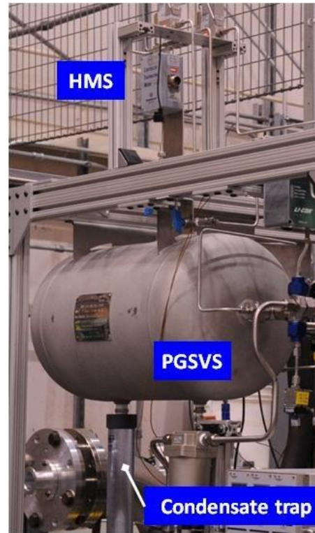
Figure 9. PGS (suit) volume simulator with HMS attached.
